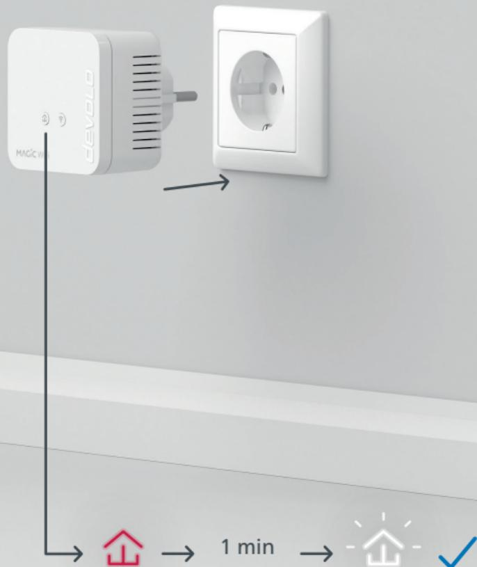
**| EN |** Connect the devolo Magic WiFi mini adapter to a free wall socket and wait until the 🏠 LED quickly flashes white (approx. 1 minute).
