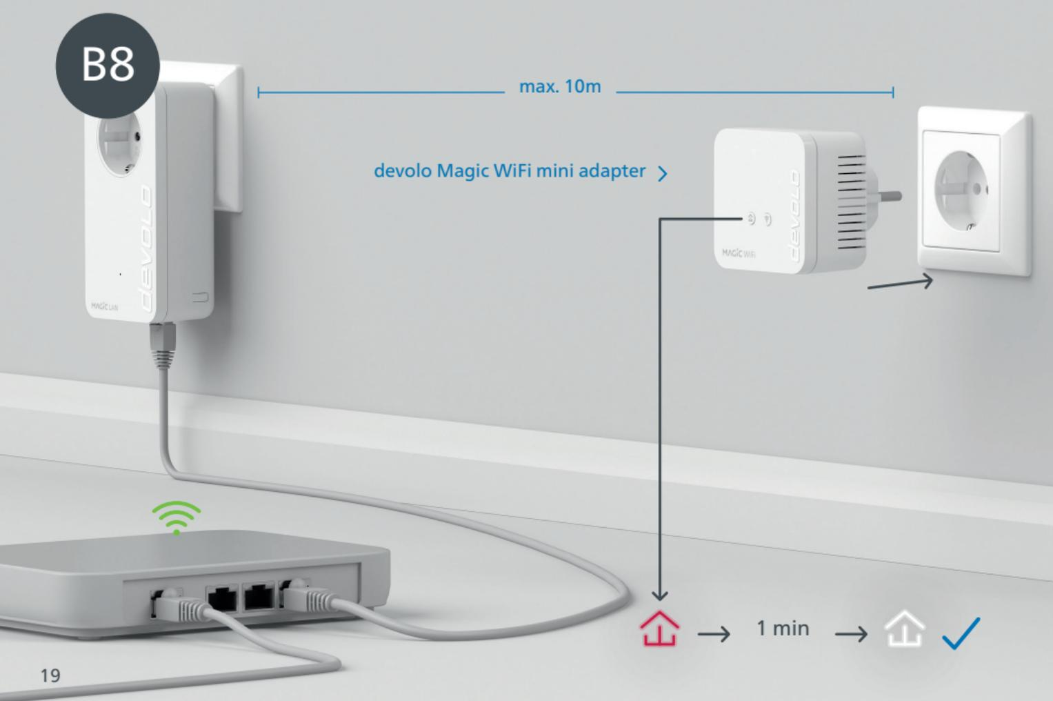
**EN** | Connect the devolo Magic WiFi mini adapter for the transmission of the Wi-Fi access data to a free wall socket near your router (max. distance 10 metres) and wait around 1 minute until the
